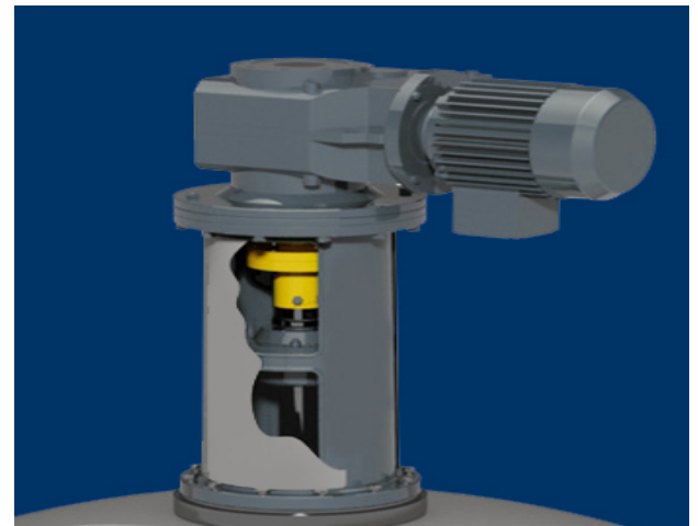
Top entry mixer with pedestal bearing and double mechanical seal. This pedestal includes a special jacket that allows for the seal to be removed without requiring external rigging - no lifting crane nor forklift required.
