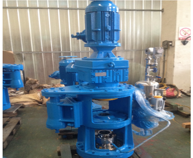
Top entry mixer with pedestal bearing and double mechanical seal. This pedestal includes a special jacket that allows for the seal to be removed without requiring external rigging - no lifting crane nor forklift required.
